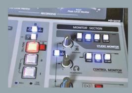
Advanced monitor panel with 5 channels allows the independent management of 4 stereo outputs for Studio and Control loudspeakers and headphones.
