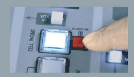
The cell phone line is wirelessly operated via Bluetooth with digital audio connection achieving a better sound quality.
