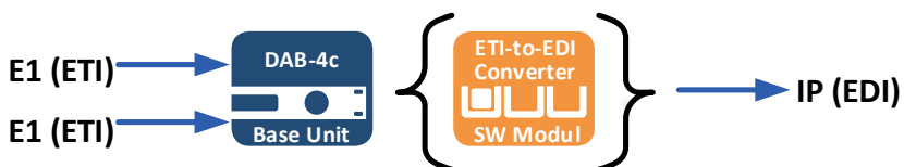
ETI-to-EDI converter with ETI Redundancy
