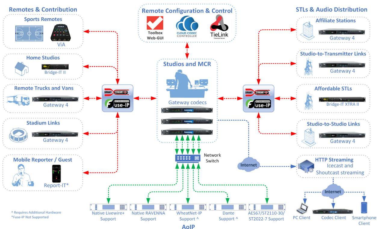
Multiple streaming solutions offered by Gateway multichannel codecs.
