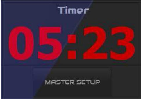
The timer start the count from 00:00 when a microphone channel turn ON, so the conductors can monitoring their adverts time.
