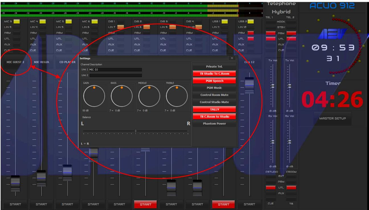
For each channel it is available the channel setup function, this mask include all setup of the hardware functions: the GAIN and Tone Control can to be modify the value with the rotation of the virtual potentiometers
