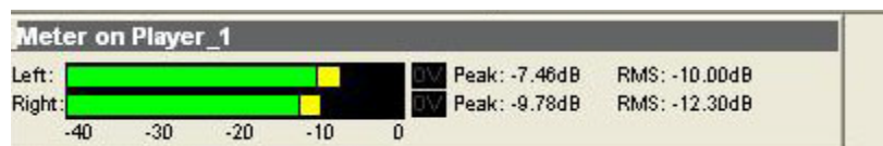
Figure 3. A stereo peak meter display. The RMS is the green bar and the peak is the yellow bar.
