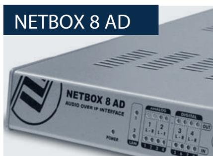
Netbox 8 AD provides 8 local input and output channels that can be connected to the NETBOX 32 AD MX through the AoIP network. I/O's are available in 4 mono analogue and 2 digital stereo channels. The second digital stereo interface can be switched for a USB connection. It also offers 4 GPI /O's that can be transported between different AEQ devices using Virtual GPIO over IP.
